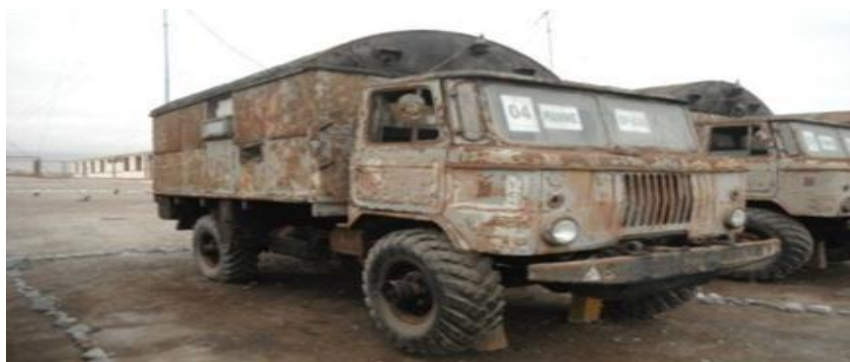
Figura 8. Cabina de radio relay
